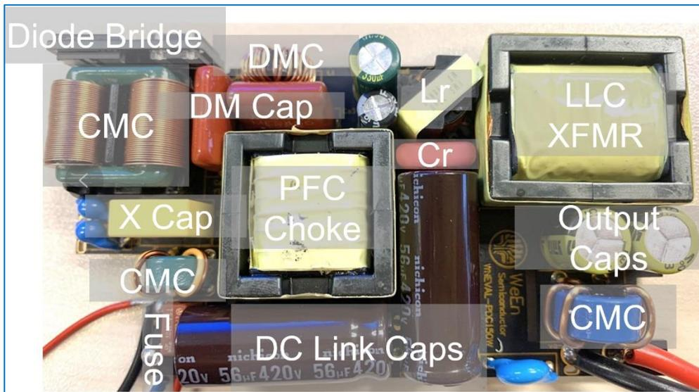
Fig. 7. PD charger reference design- PCB top view
