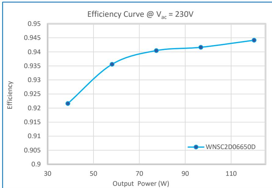
Fig. 12. Efficiency curve (230V)
