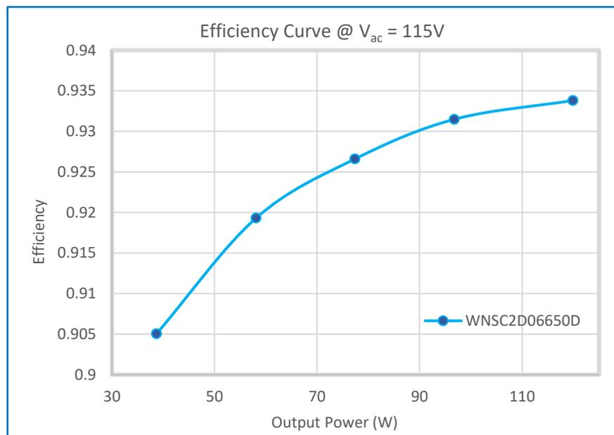
Fig. 11. Efficiency curve (115V)
