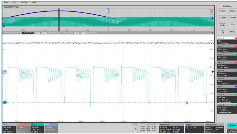
Fig. 10. DCM mode PFC Boost @ 230Vin, 400Vout, 120W, 110kHz
