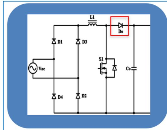
Fig. 2 Typical PFC boost circuit
