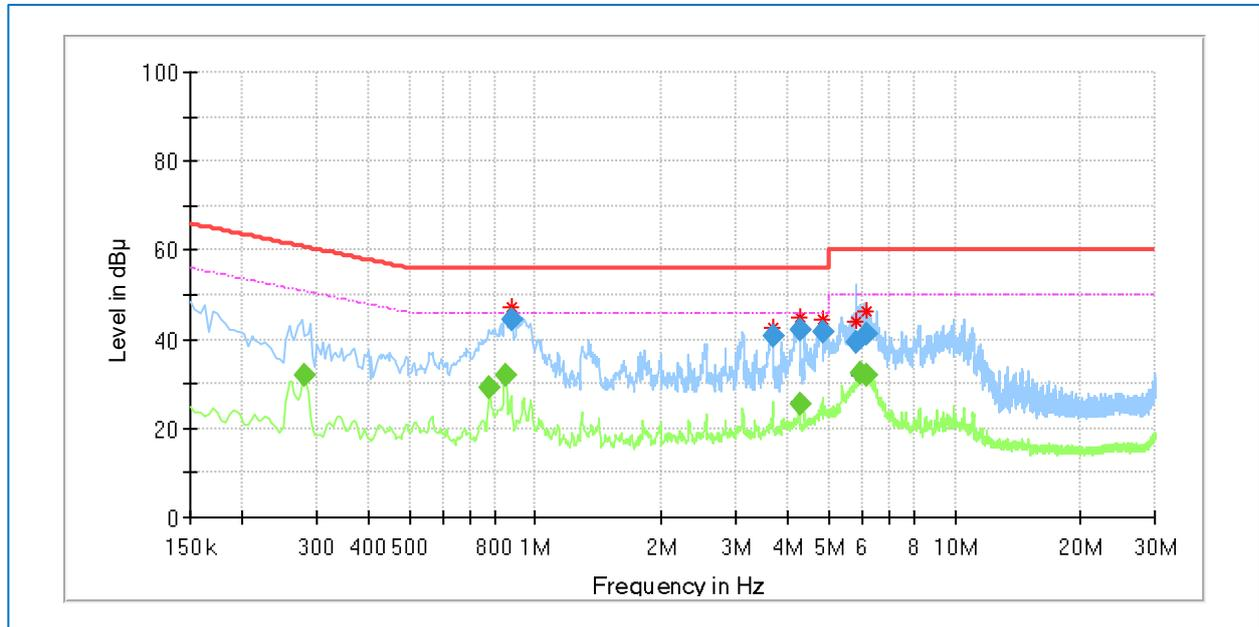
Fig. 17. Conducted EMI (Quasi-Peak blue, AVG green,  $V_{in} = 230V_{ac}$ ,  $P_{out} = 120W$ )
