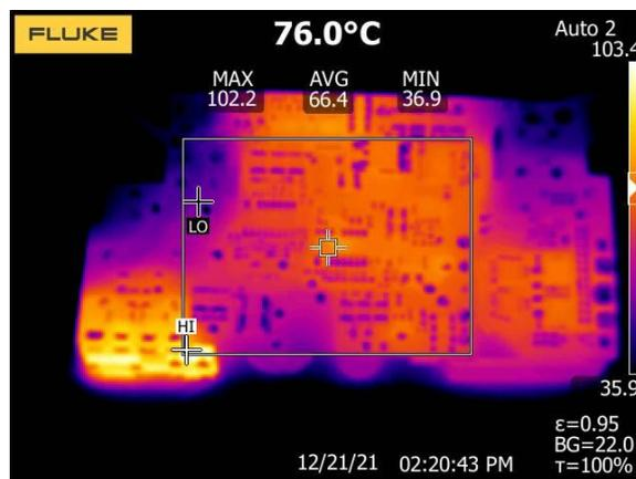
Fig. 16. PCB bottom @ 90Vin, 120W full load, open frame and no cooling
