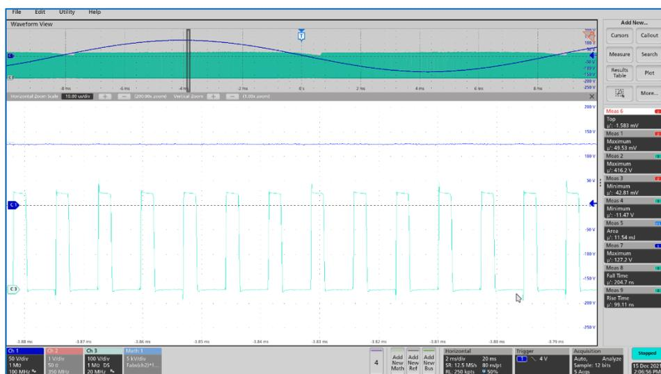
Fig. 9. CRM mode PFC Boost @ 90Vin, 400Vout, 120W, 140kHz
