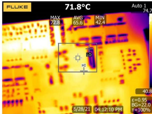
Fig. 14. WNSC2D06650D 71.8°C @ 90Vin, 120W full load, open frame and no cooling
