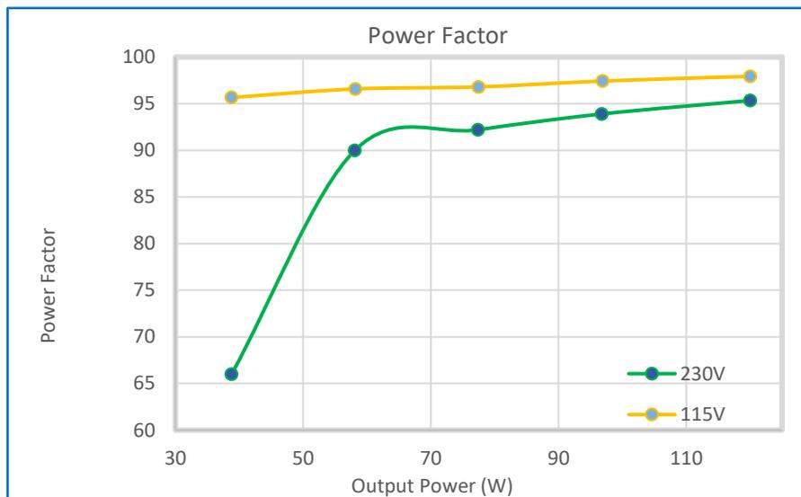
Fig. 13. Power factor curve
