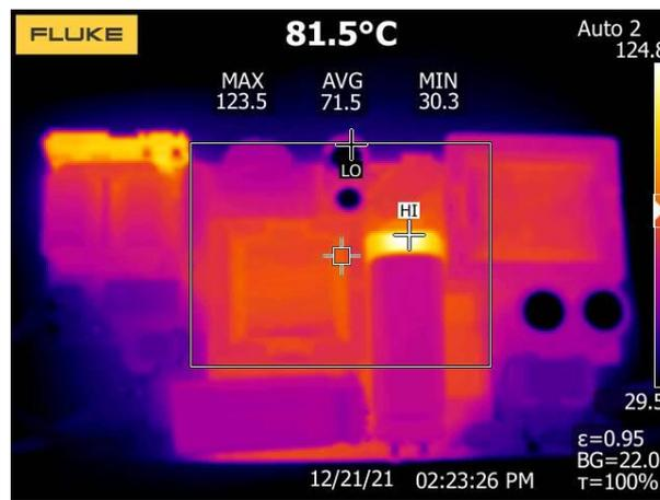
Fig. 15. PCB topside @ 90Vin, 120W full load, open frame and no cooling
