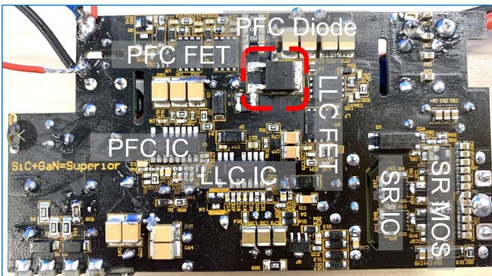
Fig. 8. PD charger reference design- PCB underside view
