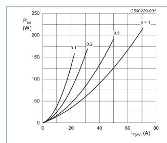
$$\begin{split} & I_{\text{F(AV)}} = I_{\text{F(RMS)}} \times \sqrt{\delta} \\ & V_{\text{o}} = 1.189 \text{ V; R}_{\text{s}} = 0.0263 \text{ }\Omega \\ & \text{Fig. 1.} & \text{Forward power dissipation as a function of average forward current; square waveform; } \\ & \text{maximum values} \end{split}$$
