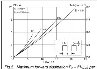
Fig.5. Maximum forward dissipation  $P_F = f(I_{F(AV)})$  per diode; square current waveform where  $I_{F(AV)} = I_{F(RMS)} \times \sqrt{D}$ .
